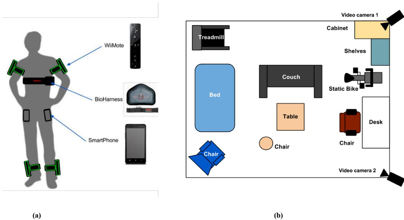
Figure 1. a) Sensing platform. B) Sensing environment, including the view of the two cameras recording the study.
